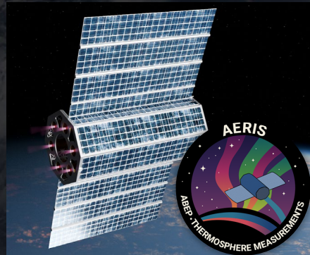
Figure 3: Blue Team's runner-up VLEO satellite mission design AERIS - Air-Breathing Electric Propulsion for Research in the Ionosphere and Thermosphere Satellite, presented at the international Satellite Design Workshop 2025.
